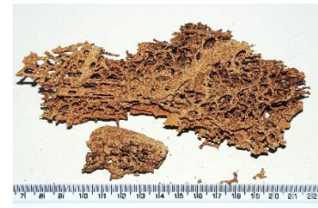
16 Termite damage removed from ceiling
